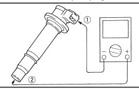
Measure the secondary coil resistance.
