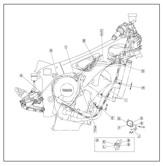
L Clamp the clutch cable by routing the upper end of the clamp along with the bottom end of the hose clamp assembly.
