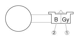
Measure the crankshaft position sensor resistance.
